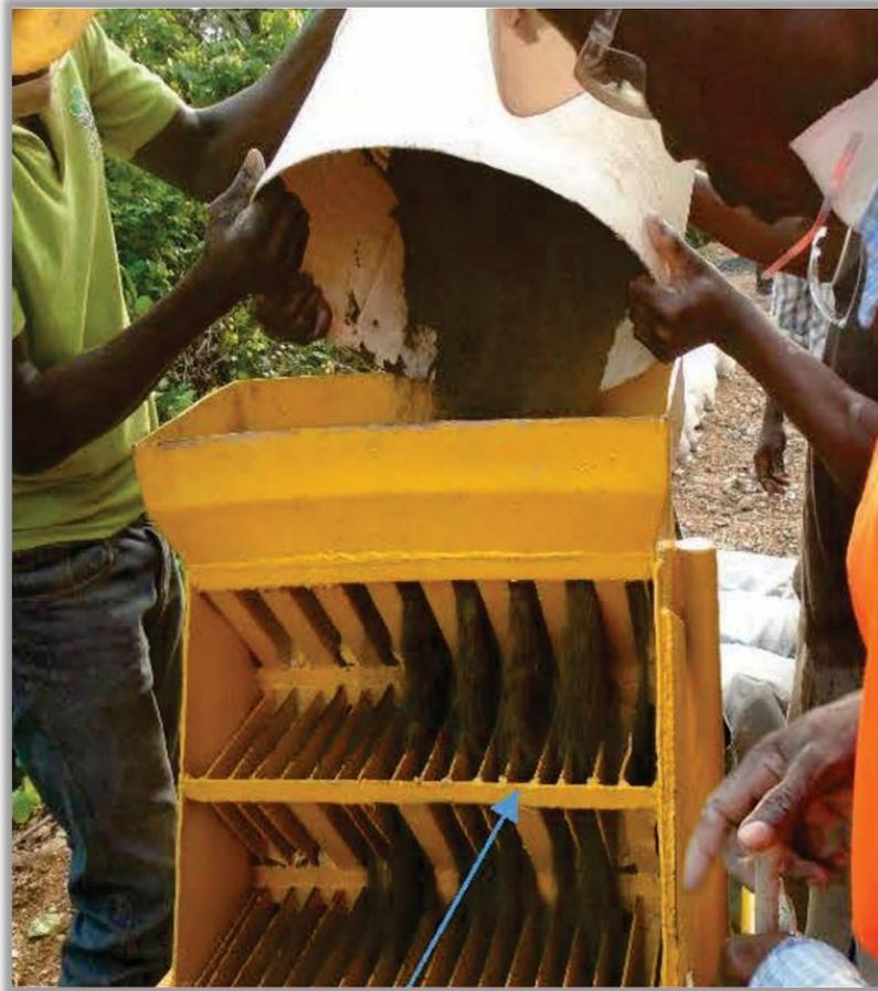
**Figure 10-23: Reverse Circulation Sampling Riffle Splitter (Newcore, 2017)**
