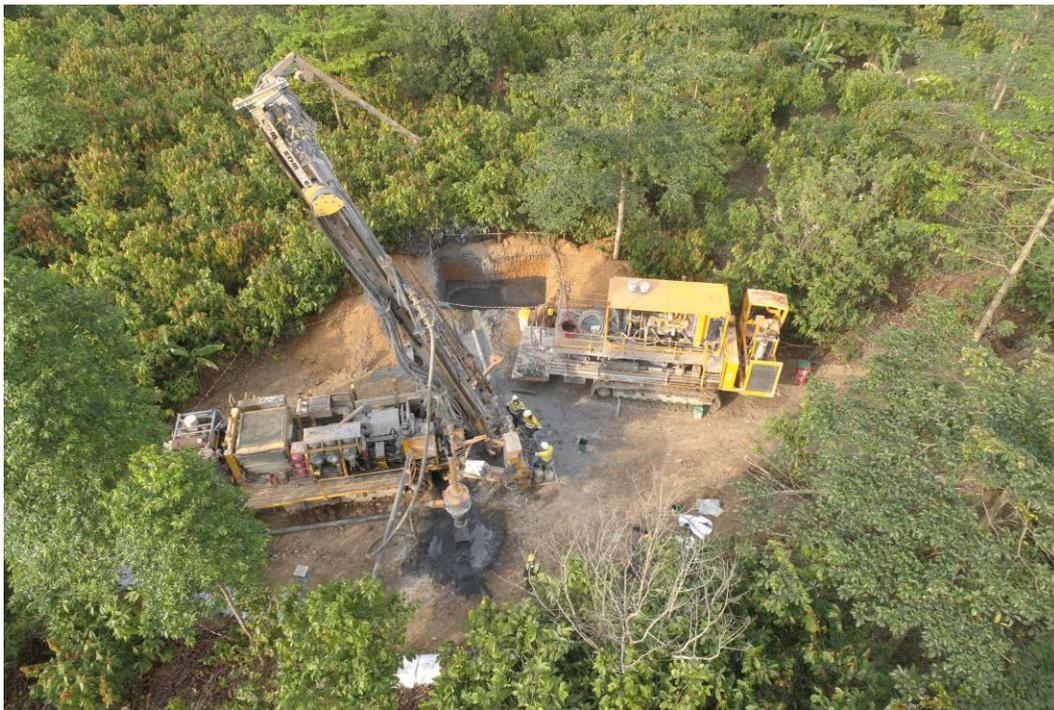
Figure 10-17: Reverse Circulation Drill (Newcore, 2021)
