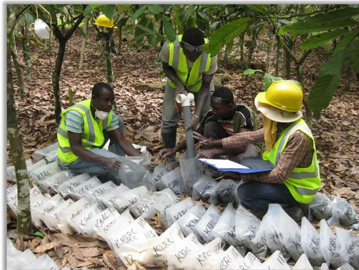
**Figure 10-22: Reverse Circulation Sampling Using Tube Splitter (Newcore, 2012)**
