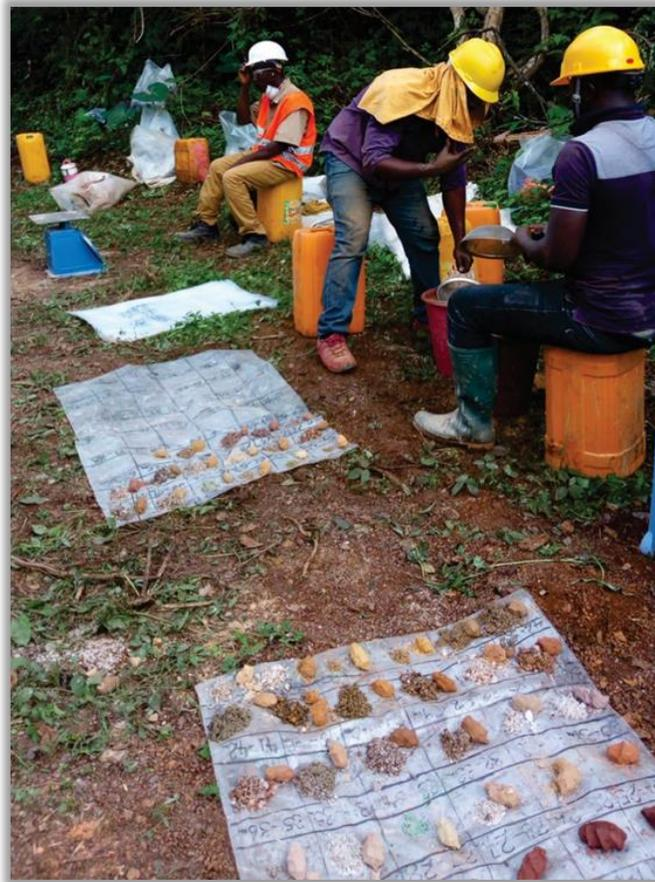
Figure 10-19: RC Chip Logging (Newcore, 2017)
