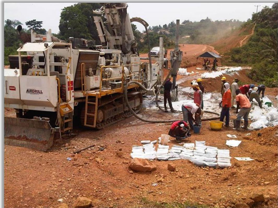
**Figure 10-1: Reverse Circulation Drill (Newcore, 2012)**
