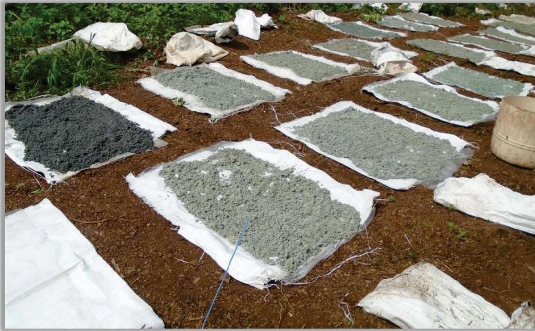
Figure 10-24: Drying Wet RC Samples (Newcore, 2017)
